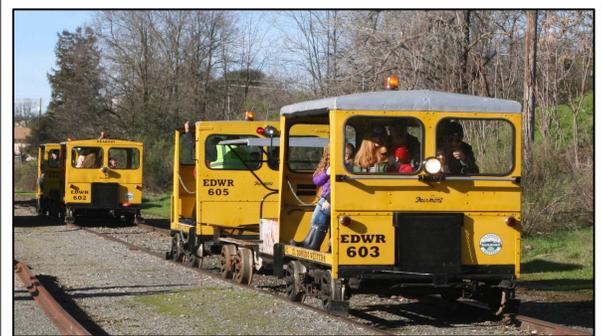
**Speeder Cars**—also known as "Gang Cars," "Inspection Cars" or "A-Cars"—were rail vehicles used to transport maintenance workers, track inspectors and assorted railroad ruffians for over 100 years from the late 1880s to the early 1990s. Unique in their own right, the gasoline-powered Speeder Cars have developed quite a following of devoted fans.
